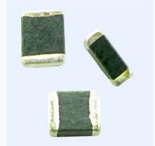
The ZVE is available in standard 0603, 0805, 1206, and 1210 chip sizes. Operating voltage is 18 Vdc and clamping voltage is 50 volts at 2 amps. Capacitance ranges from 75 pF on the 0603 size to 400 pF on the 1210 size product. The surface mount ZVE series is available in standard 7" tape and reel packaging. Pricing varies with size and ranges from \$0.085 each to \$0.185 each in full reel quantities. Contact Stackpole volume pricing.
