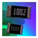
In addition to the value range expansion, the RNCF Series is also available in 0201 case size down to 0.5% tolerance and  $\pm 25$ PPM (49.9 $\Omega$  to 5K $\Omega$ ). Finally as the applications that require low temperature coefficient resistors continue to climb, so do the demands for precision resistors. To address this demand, Stackpole has expanded RNCF series TCR range down to  $\pm 5$  PPM for 0402, 0603, 0805, 1206, 1210, 2010 and 2512 case sizes.
