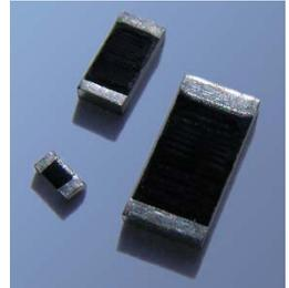
Full resistance range for the UHV Series is from 100 Megohm up to 10 Gigohm in TCR of 100 ppm and tolerances as low as 1%. The UHV typically offers untrimmed resistive elements for 10% tolerances and wider which provide the best stability over life testing and extremely low VCR. The outstanding working voltage ratings for the UHV are as follows:
