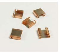
The HCSK2725 is readily available in the 1 milliohm resistance value. Other resistance values are possible based on customer demand. It is suitable for sensing currents up to 70 amps. The high temperature capability, accuracy, and stability are ideal for applications including power modules, frequency converters, motor controls, hybrid power current sensing, E-scooters, and automotive engine controls.
