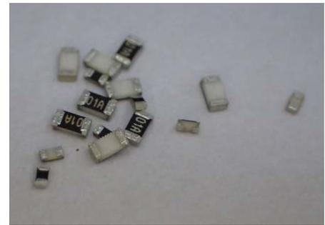
The RTAN is available in tolerances as low as 0.05% and TCR as low as 10 ppm. This precision robust performance is an ideal choice for instrumentation, aerospace, test equipment, industrial controls, portable communications diagnostic equipment, and portable medical devices.
