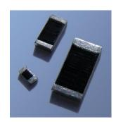
The UHV Series is available in case sizes ranging from 2010 to 5020. Tolerances are available down to  $\pm 1\%$  and TCR down to  $\pm 100$  ppm/°C. Resistance values for the UHV series range from 100 Meg  $\Omega$  up to 10 Gig  $\Omega$ . Stackpole has 500 M  $\Omega$ , 1 G  $\Omega$ , and 2 G  $\Omega$  are in stock. This series is ideal for use on the high voltage divider networks or any application with space constraints and high voltage requirements.
