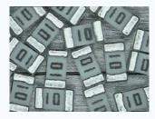
The CSRF is now available in sizes from 0402 up to 2512. Values range from 3 milliohms to 100 milliohms and in tolerances as low as 1%. Pricing varies with size, resistance value, and tolerance, and ranges from \$0.07 to \$0.30 for the most common values and sizes in full package quantities. Contact Stackpole or one of our franchised distributors for volume pricing. Current lead-times are 8 weeks. Many popular values for the CSRF are in stock or planned for stock.
