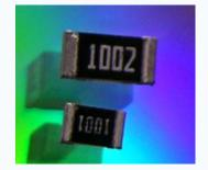
The RNCS is available in sizes from 0402 to 2512, in resistance values ranging from 10 ohm to 1Meg ohm. This series offers tolerances down to 0.1% and TCR's as low as 15 ppm / C for a limited value range. Pricing is size, resistance value, tolerance, and TCR dependent and ranges from \$0.016 to \$0.23 each in full reel quantities. Contact Stackpole or one of our franchised distributor partners for volume pricing.
