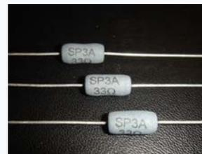
The SP3A UL recognized part (file no. E344795) is available in resistance values from 10 ohms up to 100 ohms. Other non-UL recognized values and sizes maybe available. Contact the factory for more information. Pricing for the SP3A ranges from \$0.18 to \$0.25 each in full reel quantities. Contact Stackpole or one of our franchised distributors for volume pricing. Samples are available via online distribution.
