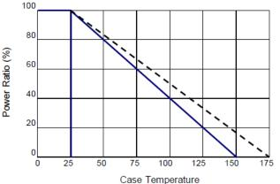
Another aspect of the power rating is the temperature at which heat dissipation is measured. Many resistors are rated at temperatures of at least 70°C. This means the part can handle the designated power rating provided the ambient temperature around the part does not exceed 70°C. However, there are some higher power resistors that are only rated for full power operation up to 25°C. These power resistors typically require some type of external heat removal to operate at full rated power.
